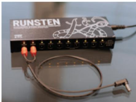
To increase the CURRENT use the DC1-48 90/0 PAR cable included with the Runsten. Connect the two Black contacts that are close together to two outputs on the RUNSTEN, and the total Current will be the sum of the two connected outputs to deliver up to 1800 mA.
