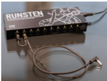
*Use this cable if the DC power input on your pedal has a 2.5 mm plug. Connect the BLACK contact to the RUNSTEN and the GRAY to your pedal.*
