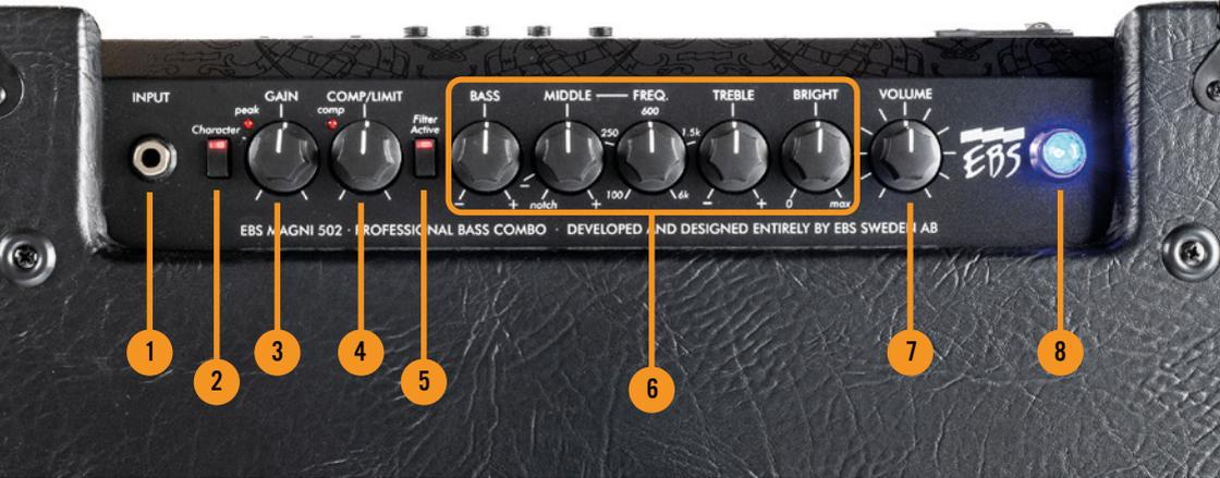
**1. INPUT** -A low noise, high impedance instrument input that will interface with passive and active instruments perfectly.
