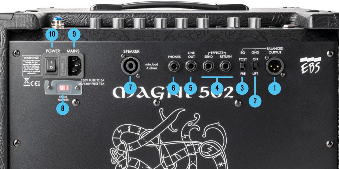
**1. BALANCED OUTPUT** -A balanced output functions as a high quality line box for connecting to PA mixing consoles or to studio or broadcast recording units, with high noise immunity. The volume level does not effect this output.
