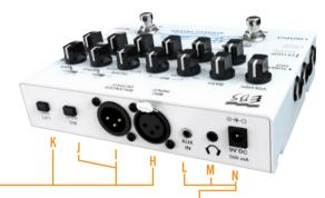
Note: The balanced output offers highauality 'line box' signal for connecting to PA mixing consoles or to studio or broadcast recording units, with high noise immunity. The output level controlled by the MASTER knob does not affect this output.
