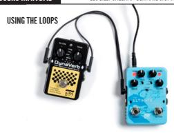
The Billy Sheehan Ultimate Signature Drive pedal gives you the option to use additional effects to affect either the Clean or Drive channel independently (the photo shows a reverb connected to the Drive Loop).
