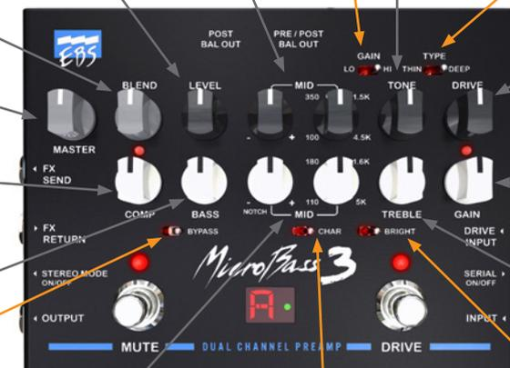
MID. These two knobs works in conjunction. Use the right control to pick a frequency. Use the left control to boost or cut the gain in the range of the chosen frequency. **Note:** When the left control is set to *Notch*, you can use the right control to find and erase a precise frequency that causes unwanted feedback (a common issue with upright basses in larger rooms).
