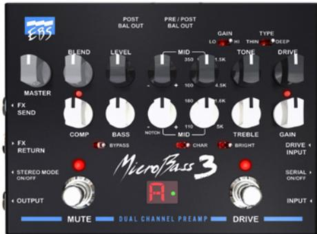
**E** DRIVE INPUT. This input is a direct input to the Drive channel in parallel mode and can be used to mix two sources, e.g. between two pickups on an instrument where applicable. Note: In conjunction with the *Blend* knob at max, and by choosing the *LO* gain engine (and modest or minimum *Drive* setting) it can serve as an input for a second instrument. Then you will use the drive channel to tweak the EQ individually for that instrument (not necessarily using any overdrive).
