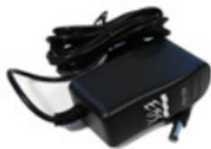
**DC POWER ADAPTOR** For environmental reasons, we recommend the use of a DC Power Supply, such as the *EBS AD-9+*. The EBS MetalDrive Studio Edition handles 9-12 V DC, and require a 2.1 mm pin center negative type of connector.
